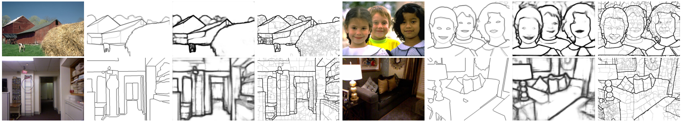
Fig. 6: Some examples of RCF. Top : BSDS500 [9]. Bottom : NYUD [36]. From Left to Right : origin image, ground truth, RCF edge map, RCF UCM map, and repeated this order.
