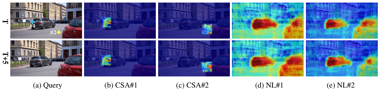
Figure 2: Visualization of the attention map produced by the non-local operation and the CSA. We query two positions (#1, #2) in frame T and get attentions of frames T and T + 5 . The non-local module produces motion-independent attention because it outputs similar attention maps for different query positions. The similar observation that the non-local module outputs query-independent attention in object detection task was made in (Cao et al. 2019). The CSA is constrained by motion prior, which focuses on motion cues.
