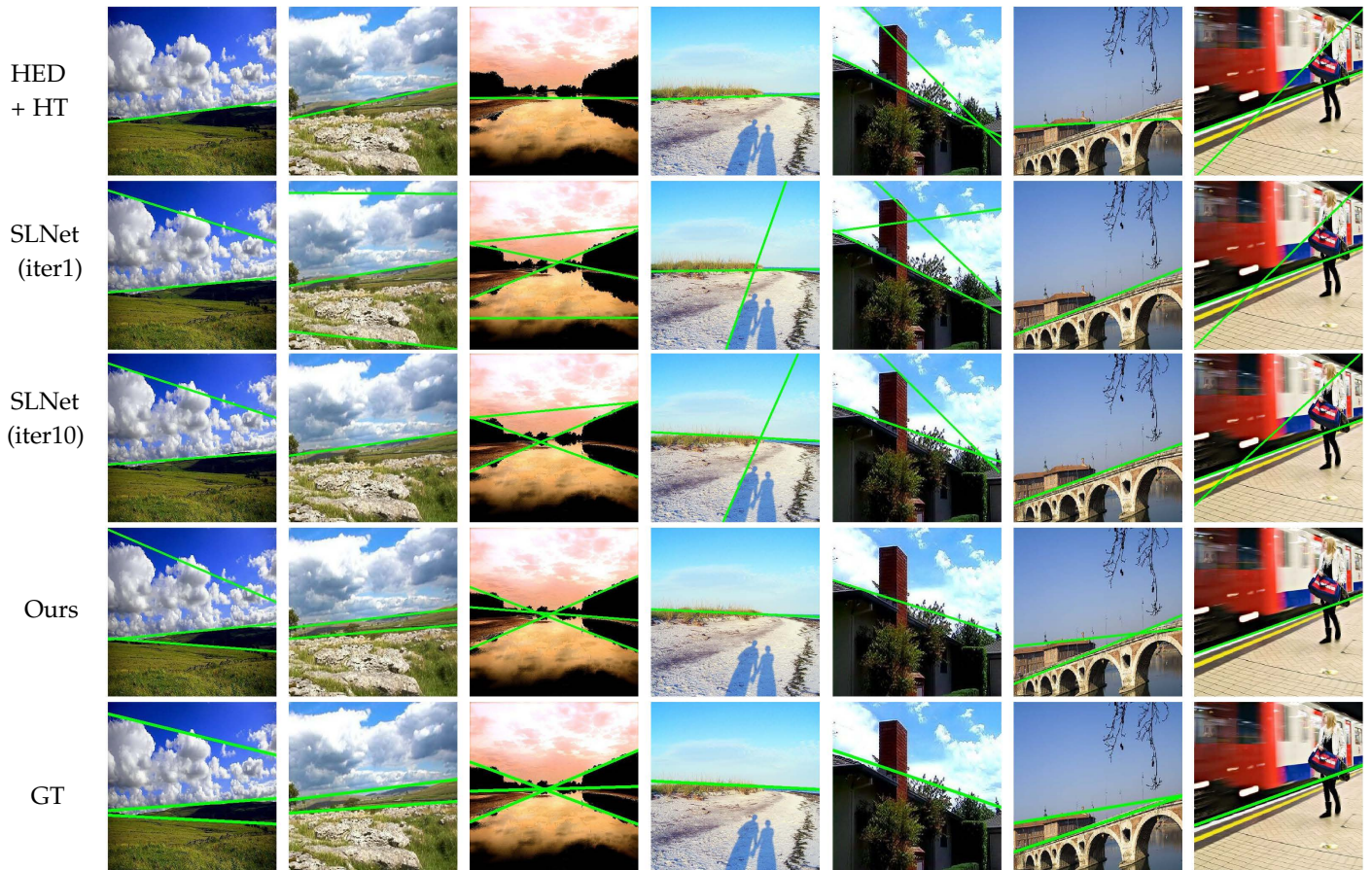
Fig. 13. Example detection results of different methods on the SEL dataset. Compared to SLNet [11] and classical Hough transform [25], our results are more consistent with the ground-truth.
