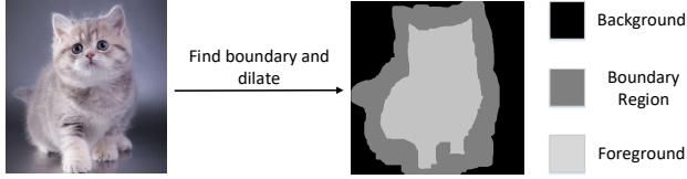
Figure 3. We dilate the boundary map and apply a binary cross entropy loss at three stages in the CNN backbone to prevent mid-level attention from drifting into boundary regions.
